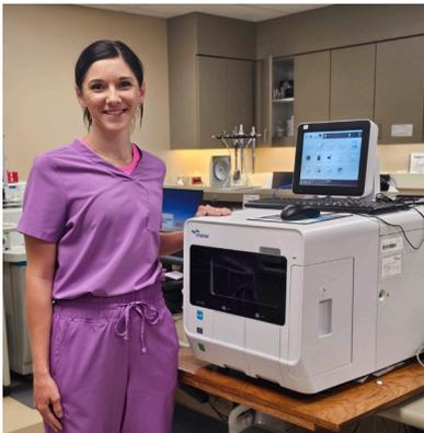
Nemaha Valley Community Hospital recently purchased an XN-550 Hematology Analyzer. This is an upgrade from the 5-part differential of our current Cell Dyn Ruby. The XN-550 is an automated compact 6-part differential hematology analyzer. It is designed to meet small size hospital laboratory needs for enhancing clinical values and improved operational efficiency.
